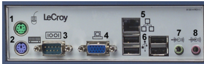
(1) Mouse 1 ; (2) Keyboard * ; (3) RS-232-C Port; (4) External VGA Monitor; (5) Ethernet Port; (6) 4 USB Ports; (7) Line In; (8) Speakers
