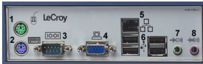
WaveMaster back panel, including the LAN port (5) used for remote control
